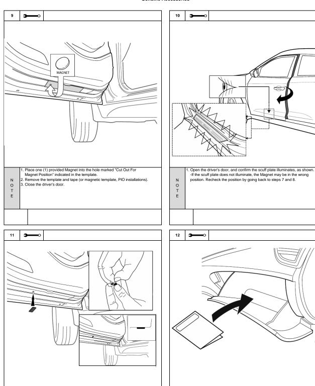
Make sure to not disturb the position of the Magnet when installing the Magnet Holder.
