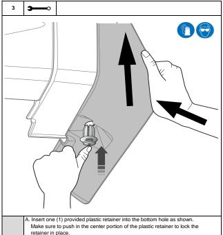
Make sure to push the mudguard upward and inward during the installation to
