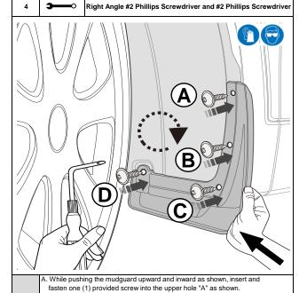
B. Insert and fasten one (1) provided screw into the middle hole "B" as
