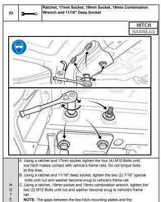
vehicle's frame rails are normal at this point in the installation. The tow hitch mounting plates will flex until they seat against the vehicle's mounting points during the hardware torquing process in the following
