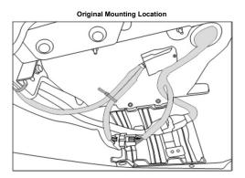
Tow hitch harness should be routed as far away from the Exhaust system as
