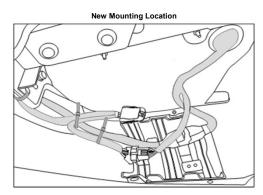
The hitch harness is located minimum 30cm (11.8") from exhaust system.
