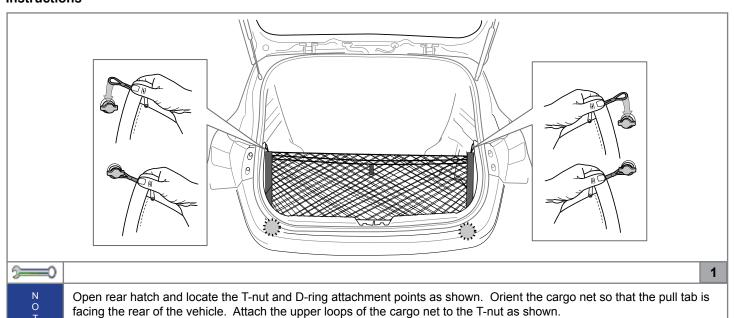
Locate the lower D-rings. Attach the plastic clips of the cargo net to the lower D-rings as shown.
