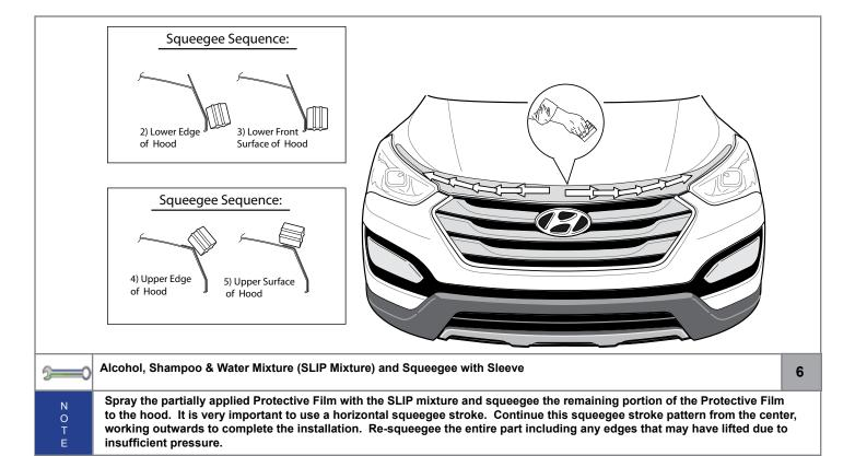
Inspect for bubbles or lifting.
