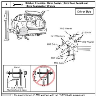
I. Pre-assemble two (2) M10 washers with two (2) M10 bolts making sure the 'toothed side' on each washer is installed facing away from the bolt head. Starting on the driver side rearmost hole, install and HAND TIGHTEN two (2) M10 bolts and washer assemblies through the hitch assembly and into the vehicle frame rail.
