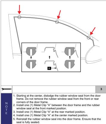
Ensure the rubber window seal is correctly seated. Be careful not to
