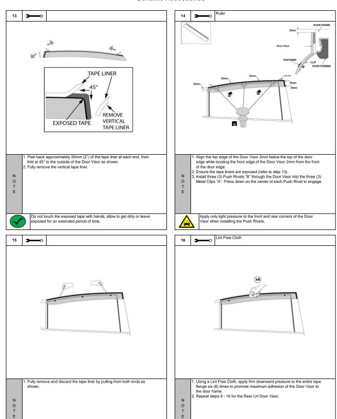
Be careful not to tear the tape liner during removal.
