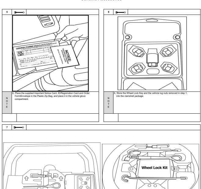
A. Place the clamshell package in the proper location near the factory lug nut wrench, typically found in the cargo area of the vehicle. Make sure the package is securely placed to avoid any rattles/noise.
