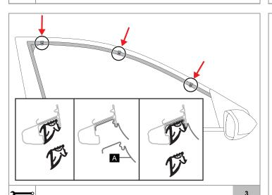
A. From the center of the upper door frame, separate the rubber window seal from the door frame. Do not remove the rubber window seal from the front or rear corners of the upper door
