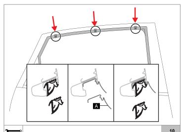
A. From the center of the upper door frame, separate the rubber window seal from the door frame. Do not remove the rubber window seal from the front or rear corners of the upper door frame
