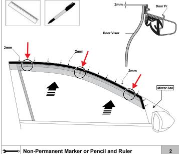
A. Remove the protective film from the Door Visor.
