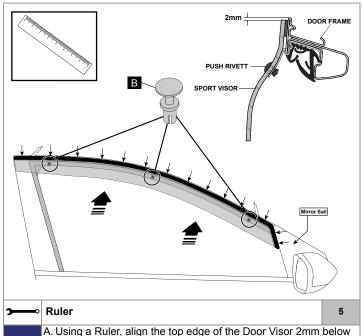
A. Using a Ruler, align the top edge of the Door Visor 2mm below the top of the door edge while locating the front edge of the Sport Visor to the inside edge of the Mirror Sail.
