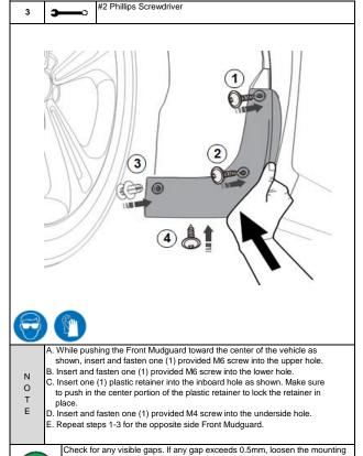
screws and refit the Front Mudguard to the body to decrease or eliminate the
